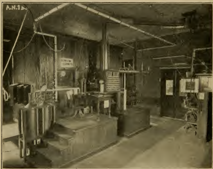
FIG. 22. — Respiration calorimeter at the Institute of Animal Nutrition, State College, Pa.
